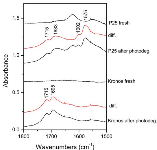
Fig. 7 Absorbance FTIR spectra relative to fresh and used P25 (top spectra) and 1077 (bottom)  $\text{TiO}_2$  samples in the ethanol degradation reaction. The differences between the spectra of the samples before and after ethanol degradation are reported in red.
